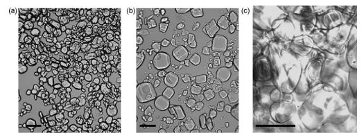
Fig. 6 – Micrographs of mirabilite crystals after  $1\tau$  (a) and after  $3\tau$  (b) {scale bar = 300  $\mu$ m}. Micrograph (c) represents the ice crystal product after  $3\tau$  {scale bar = 400  $\mu$ m}.
