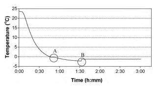
Fig. 3 – Graph showing the temperature profile for a 5 wt% Na<sub>2</sub>SO<sub>4</sub>-H<sub>2</sub>O system cooled from ambient to eutectic.
