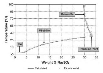
Fig. 2 – Binary phase diagram for Na<sub>2</sub>SO<sub>4</sub>-water showing regions of stable phases (Thomson, 2007).
