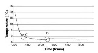
Fig. 4 – Graph showing the temperature profile for a 4 wt% Na<sub>2</sub>SO<sub>4</sub>-brine system cooled down from ambient to eutectic.
