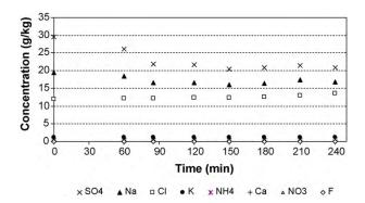
Fig. 5 – Graph showing the change in concentration of the different ions in solution for a  $4 \text{ wt}\% \text{ Na}_2\text{SO}_4$ -brine system cooled down from ambient to eutectic.
