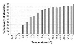
Fig. 7 – Graph showing the theoretical recovery of mirabilite with decreasing temperature.
