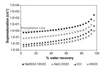
Fig. 1 – Supersaturation of various salts from the reverse osmosis retentate stream as a function of water recovery.
